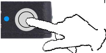
Hold **Bluetooth MFB** in at least 6 sec to reach Pairing Mode the first time a new device is connected, > 2 sec thereafter to easily connect from Idle Mode
