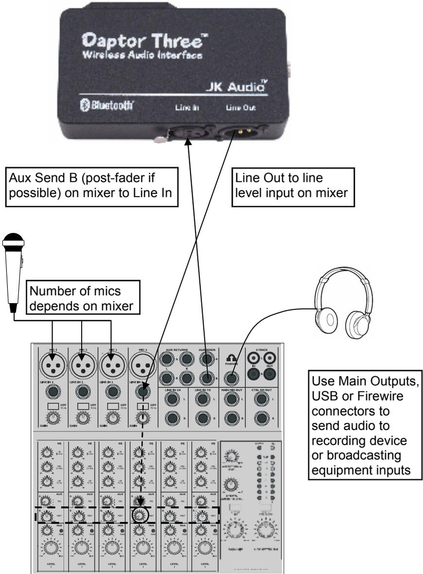
For whichever input channel you have the Caller connected to, turn the corresponding Aux B control to minimum (usually hard left) so you are not sending the caller's own audio back to them. All other Aux controls for that aux bus should be set for what you want to send to the phone caller.
